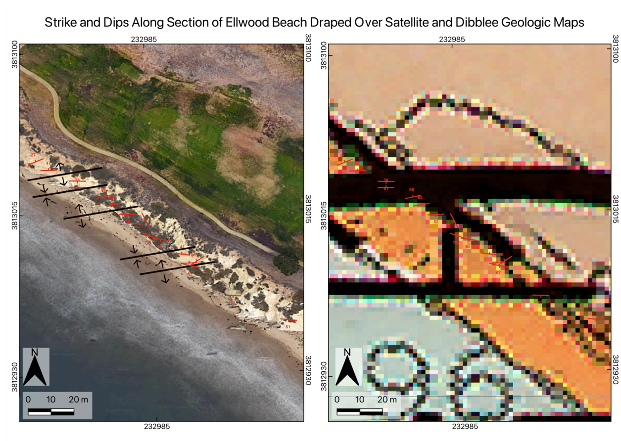
Figure 10. The red strike and dip measurements taken along Ellwood Beach overlie satellite and Dibblee geologic maps to indicate structure orientation and folding. The black fold axes overlie the satellite map to display the syncline or anticline nature of the fold.
